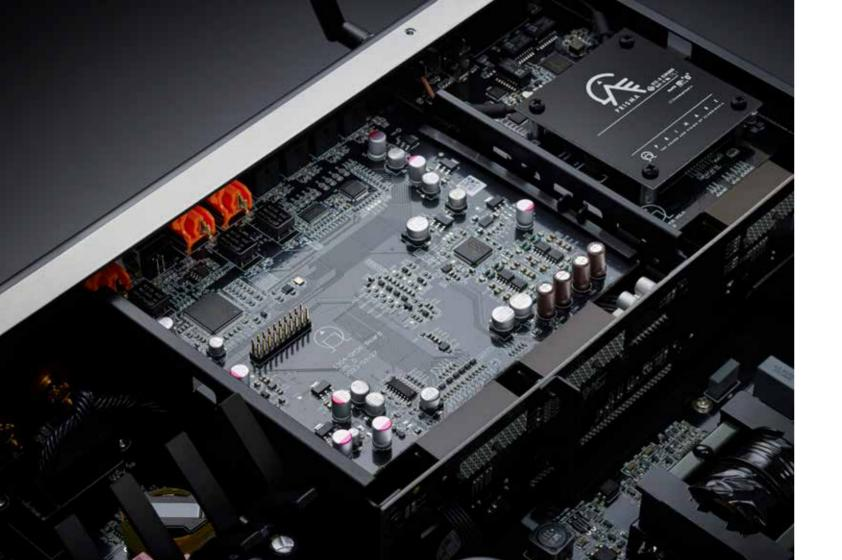
SM35 is an advanced network player module providing Prisma control and connectivity technology to CD35, I25, I35, and PRE35 platforms.
