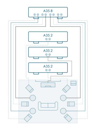
Adds three bridged A35.2 amplifiers for Front Left, Right, and Centre speakers, while the A35.8 provides the Surround Left and Right, Rear Surround Left and Right, and Front and Rear Left and Right Height speakers.
